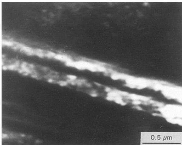
Figure 5 Dark-field transmission electron micrograph of thin strain-induced martensite laths.
