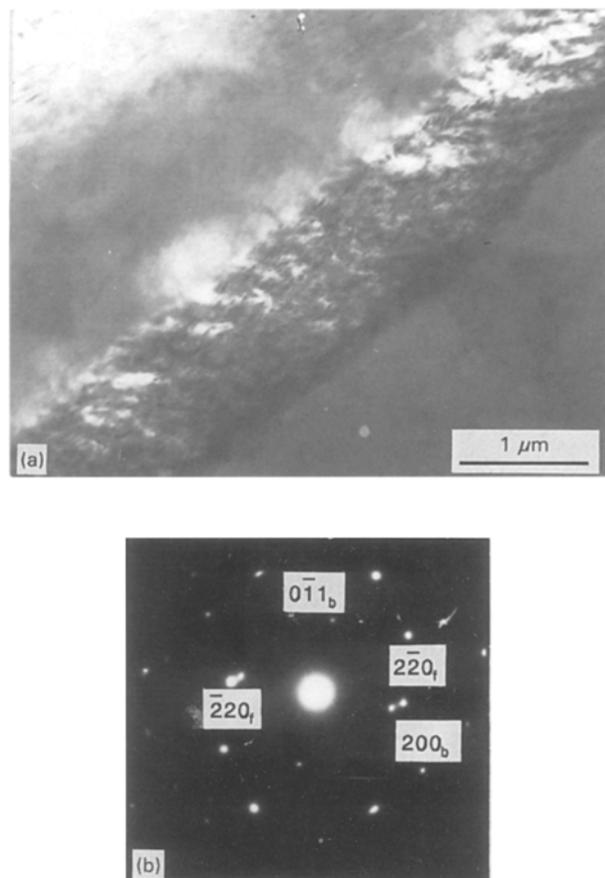
Figure 1 (a) Transmission electron micrograph of a strain-induced martensite showing a high density of dislocations. (b) Indexed selected-area diffraction pattern from the austenite–martensite interface.
