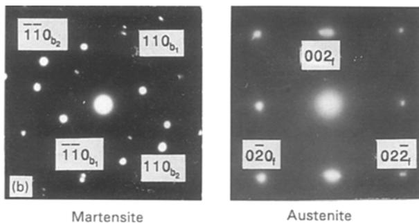
Figure 2 (a) Transmission electron micrograph of a butterfly-like strain-induced martensite. (b) Indexed selected-area diffraction patterns taken from the encircled area in (a) and austenite matrix. The twinned martensite diffraction consists of two superimposed patterns ( $b_1$  and  $b_2$ ).
