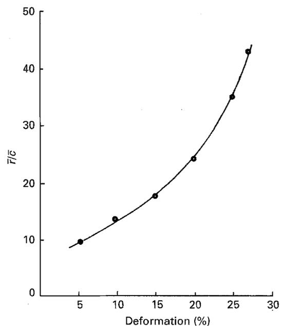
Figure 6 Mean aspect ratio of strain-induced martensites after various amounts of plastic deformation at room temperature.
