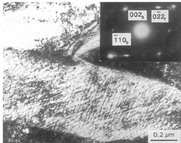
Figure 4 Transmission electron micrograph of a strain-induced martensite with a parallel array of straight dislocations and corresponding selected-area diffraction pattern.
