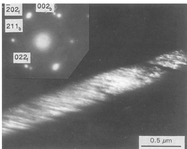
Figure 3 Dark-field transmission electron micrograph of a lath-like strain-induced martensite and corresponding selected-area diffraction pattern.
